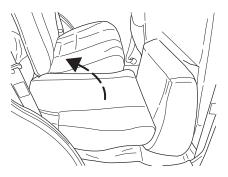
2. Rotate seat cushion down into the seating position making sure that the seat cushion is locked into place and that the safety belt buckles are exposed.
